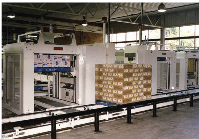
Modular line using three palletisers in an inline configuration.
