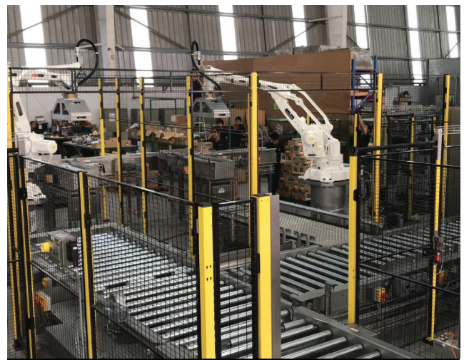
Dual robotic palletising system installed at Nestle Smithtown.
